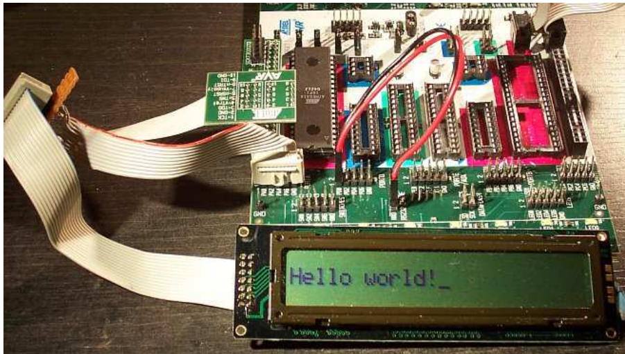
Figure 9: Wiring of the STK500
